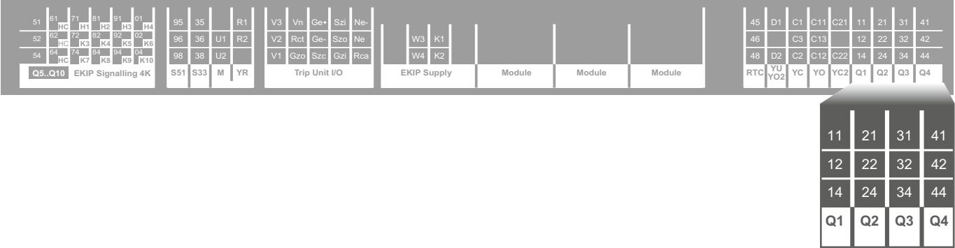
81) Open/closed auxiliary contacts of circuit-breaker - AUX 4Q (4 Form C)
